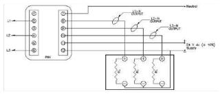
Typical 4-20 mA input to processor Max loop resistance 600 Ω/phase
