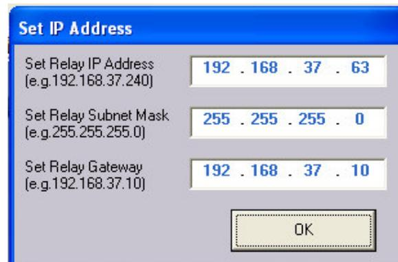
**FIGURE 9-19: IP ADDRESS SETPOINT WINDOW**
