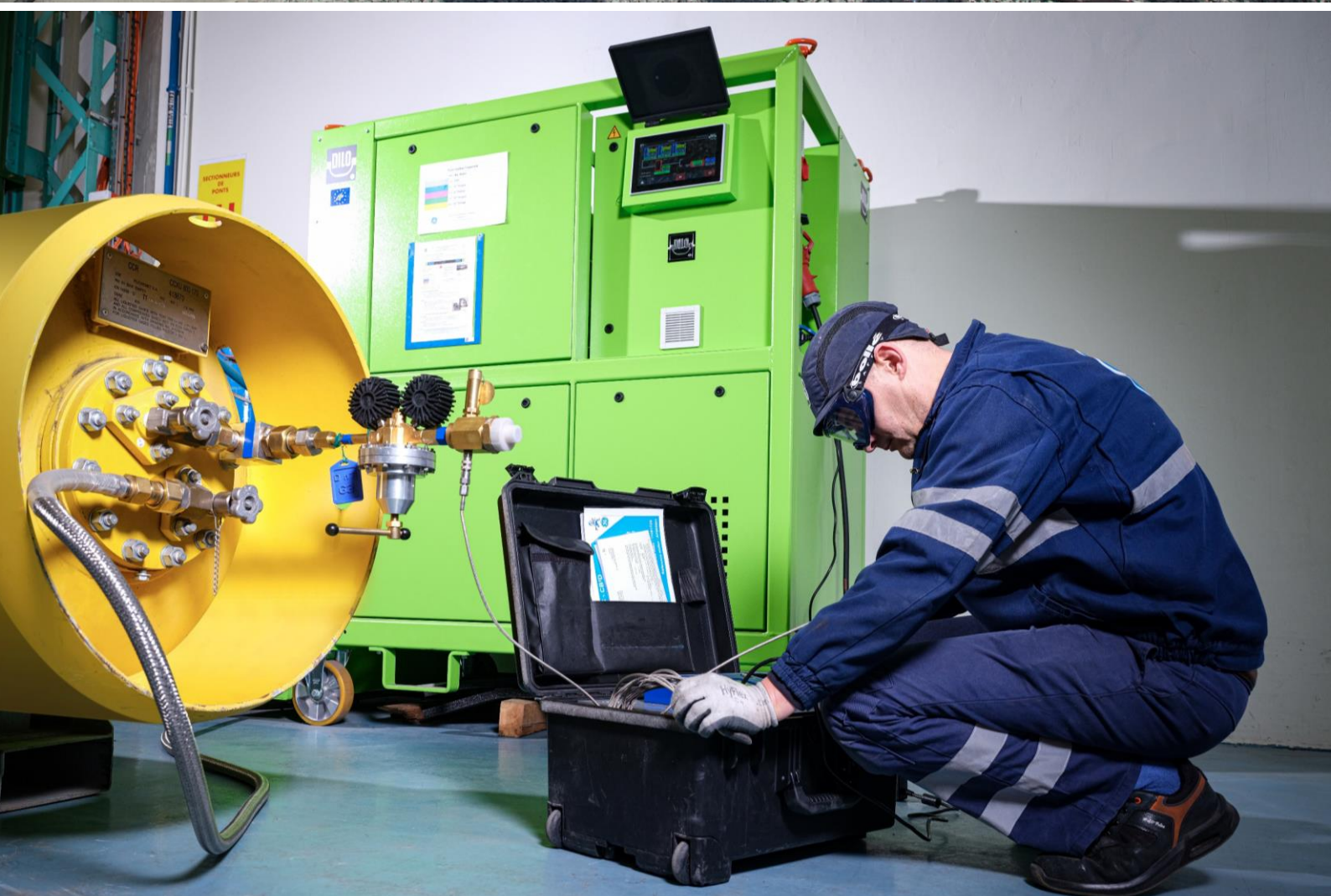
Figure 46: Gas quality routine check of a recently prepared gaseous premixed mixture using a mixing cart
