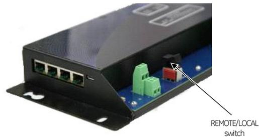
The D20E Remote/Local switch is disabled by default. To enable the remote/local switch, follow the procedure described in section: [Operation of control output points](#) on page 73, and enable **Control**. For example, the remote/local switch must be enabled for operation with the D20MX Substation Controller.
