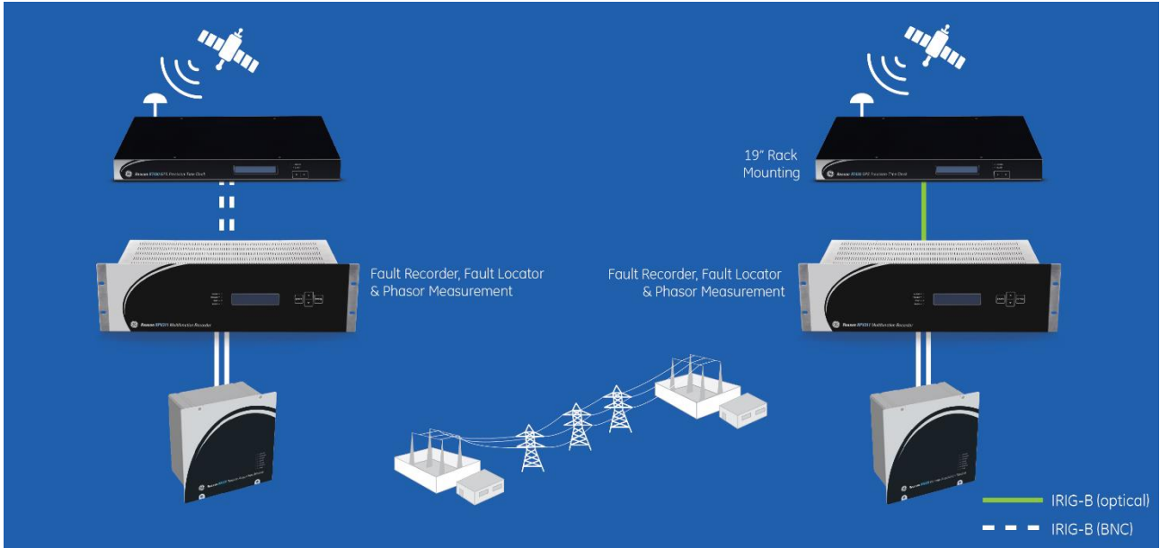
Figure 18: TWFL application using RT430/434 for Time Sync
