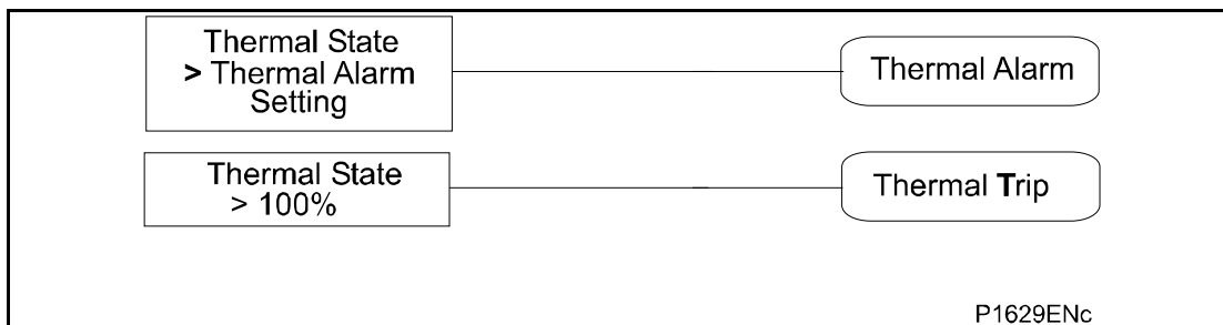
Figure 13: Thermal overload protection logic diagram
