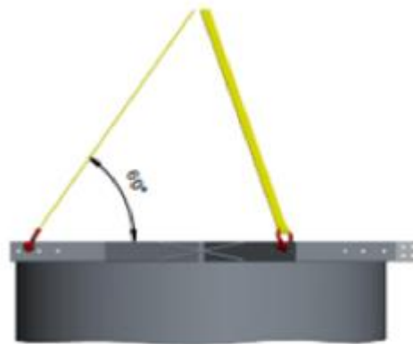
Three point lifting
