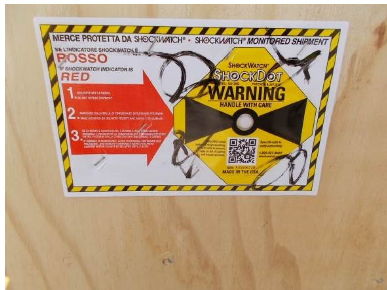
Figure 1 – Visual external shock indicator
