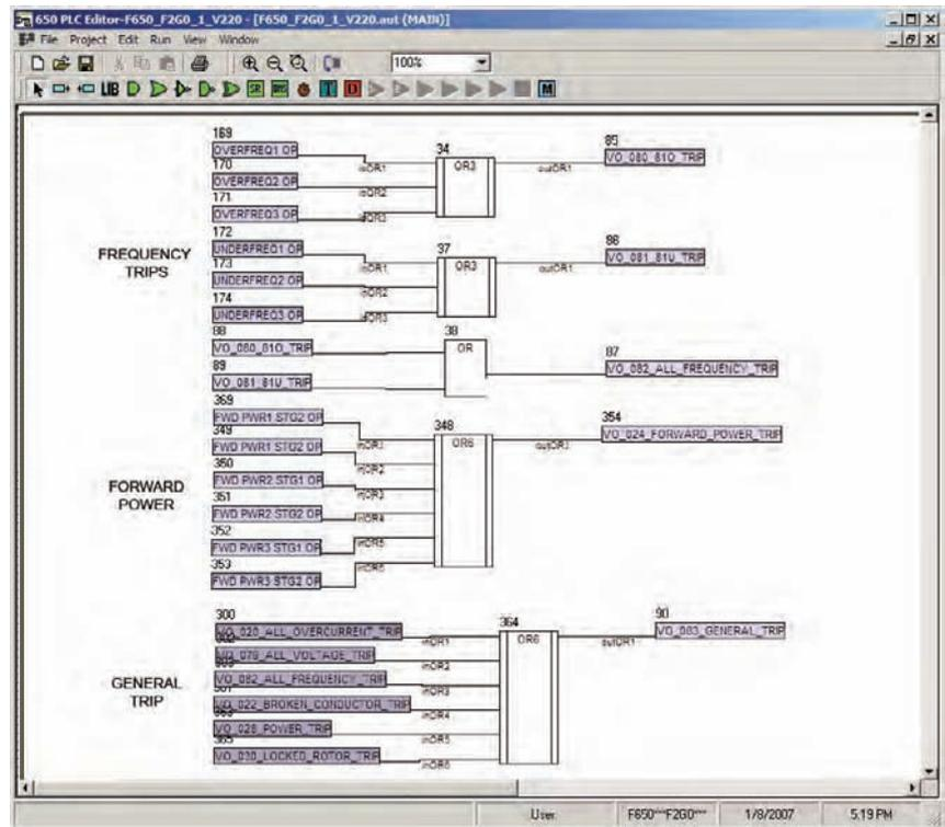
The W650 programmable control logic allows for the creation of customized wind generator protection schemes and applications.
