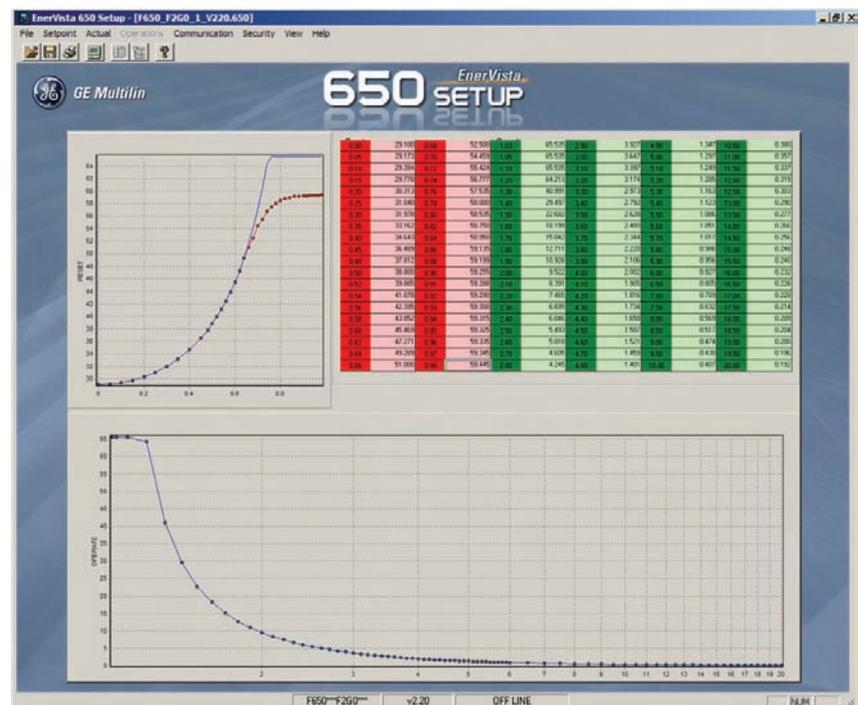
Create overcurrent curves customized to the characteristics of a wind generator using the W650 setup software
