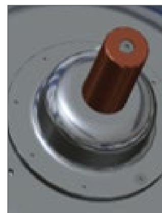
Fig. 14: top terminal conductor
