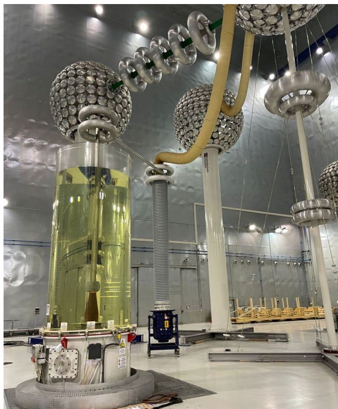
Fig. 19.1: Bushing under test
