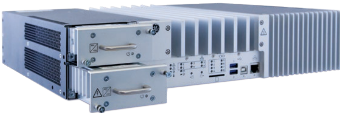
Redundant, hot-swappable power supplies.
