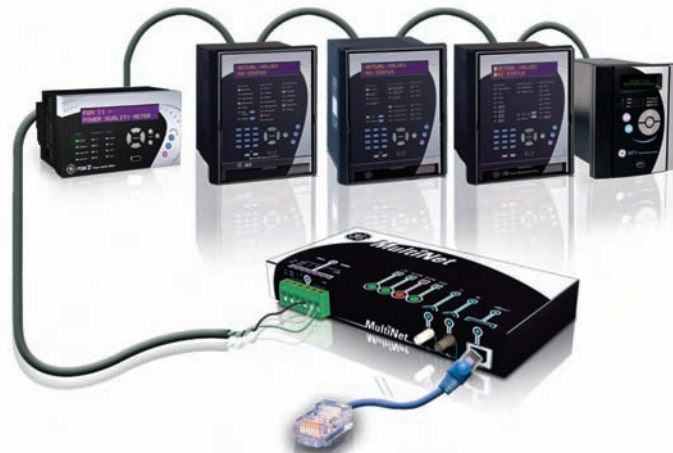
Connect up to 32 Modbus devices to your ethernet network including M II devices
