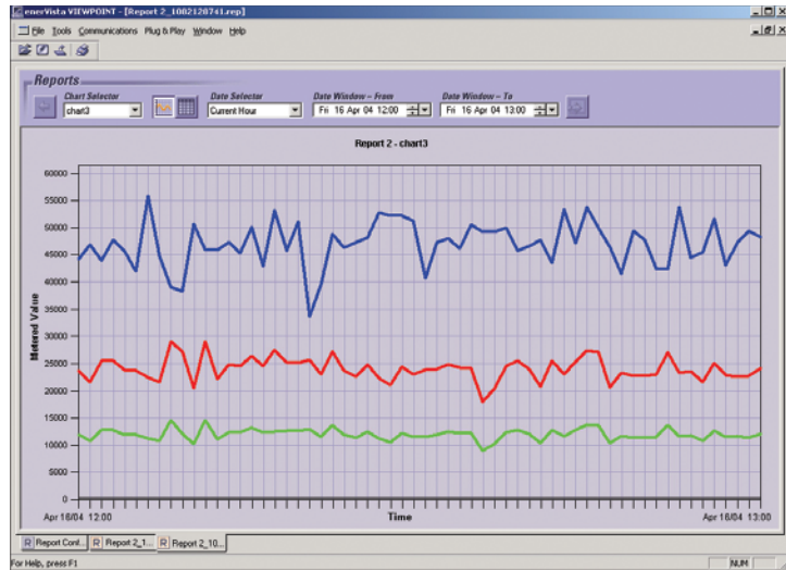
Use device software to obtain non-operational data such as trending and event records through the D400's secure remote access functionality.
