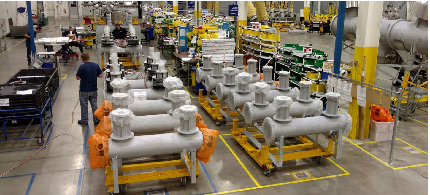
Dead Tank Circuit Breaker Assembly – installation of interrupters and current transformers to 72.5 kV dead tank circuit breakers.
