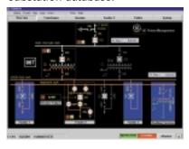
**GE-CONF** allows offline user configuration of HMI screens, databases and Level 2 functionality, including users management, access levels and passwords.
