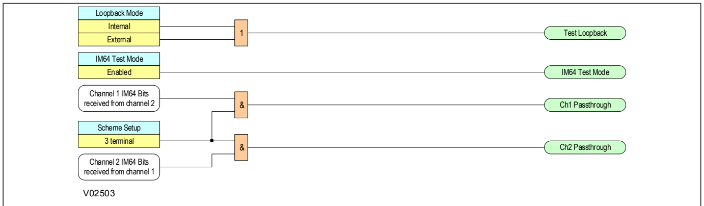
Figure 288: IM64 general alarm signals logic
