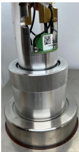
Figure 11-48: Sensor electronics piece secured in test tap adaptor piece (left) & alignment marks (right)
