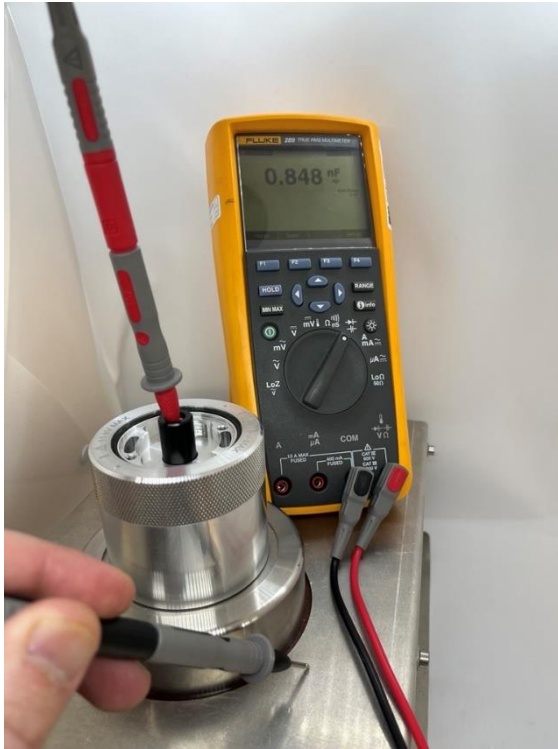
Figure 11-47: Capacitance between the test tap adaptor pin and the bushing flange
