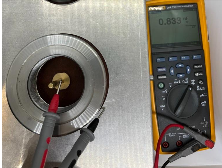
Figure 11-41: Bushing capacitance from contact pin to flange
