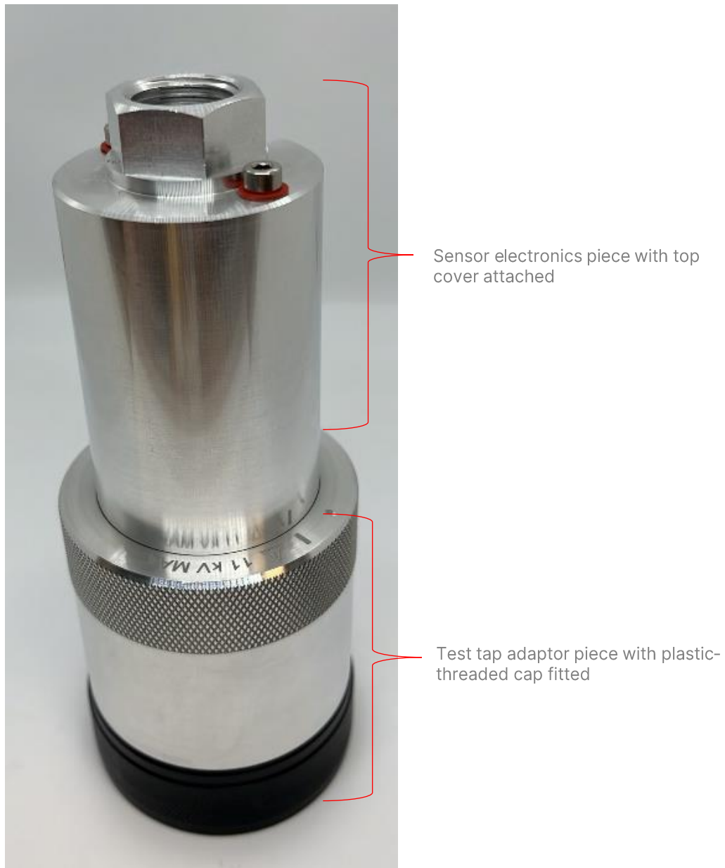
Figure 11-30: Two-piece Bushing Adaptor (vertical orientation) with plastic-threaded cap
