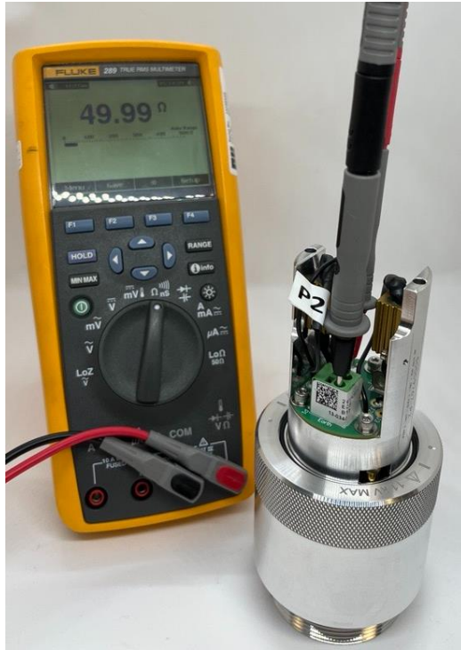
Figure 11-34: Resistance across earth and signal terminals
