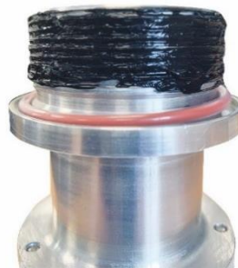
Figure 11-24: Bushing Adaptor with all threads covered in grease
