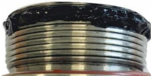
Figure 11-42: Conductive grease applied to test tap adaptor initial threads
