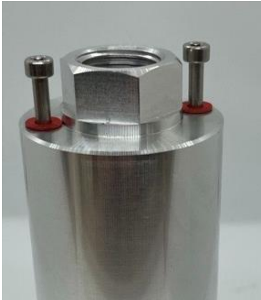
Figure 11-45: Unfasten first-threaded section of the M4 screws holding sensor electronics piece
