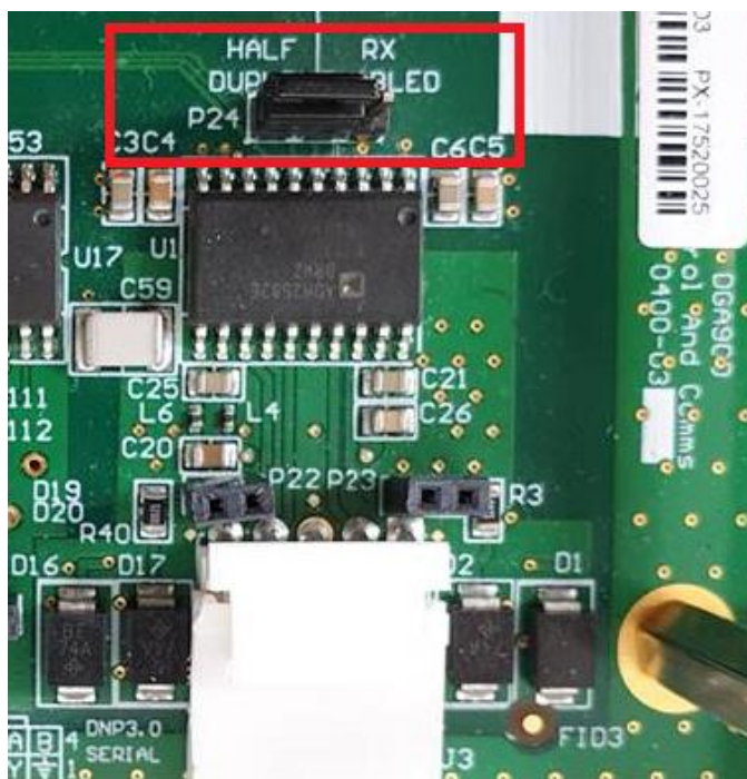
Figure 12-9: Controller board P24 jumper set to 'Half Duplex'
