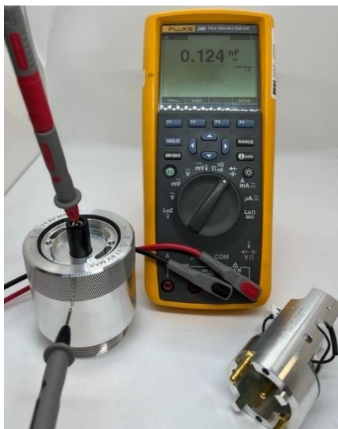
Figure 11-37: Capacitance of test tap adaptor's contact pin to its outer body
