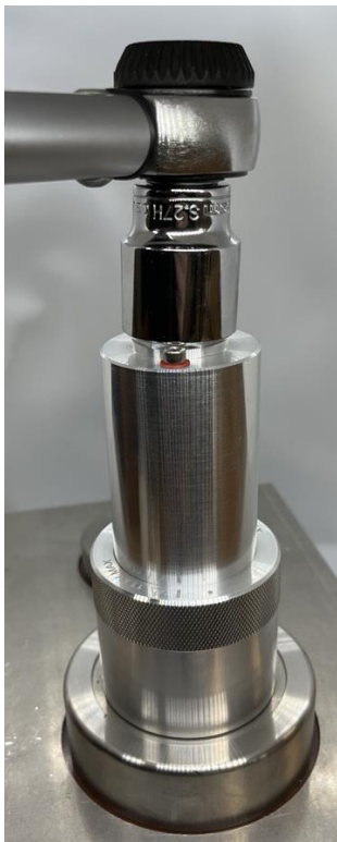
Figure 11-44: Bushing adaptor torqued to bushing tapping point
