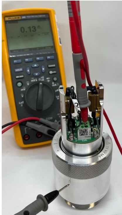
Figure 11-36: Continuity of the sensor electronics' earth terminal to the test tap adaptor's outer body
