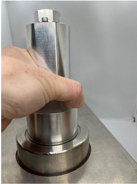
Figure 11-43: Bushing adaptor hand tight to bushing tapping point
