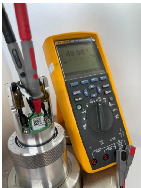
Figure 11-50: Resistance on test tap adaptor terminals
