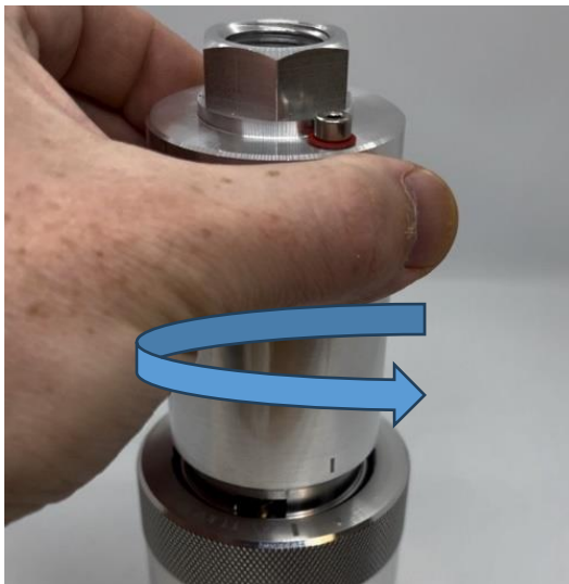
Figure 11-46: Lift & rotate the sensor electronics piece anticlockwise
