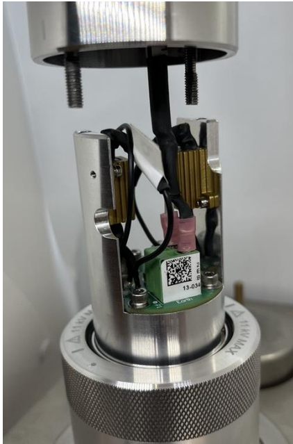
Figure 11-51: Coax cable connected through the sensor electronics top cover
