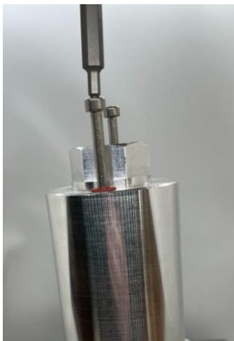
Figure 11-33: Loosen M4 screws holding sensor electronics body cover
