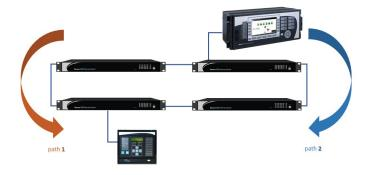
The protocol works to create a logical topology that resembles a tree. The first step is to define where the root of the tree is, in the other words, which switch will act as root bridge. The root bridge will be the logical center of the topology and the remaining switches will be designated bridges. In this setup, the remaining ports from each Ethernet switch must be defined depending on the STP protocol version used (STP, RSTP or MSTP).
