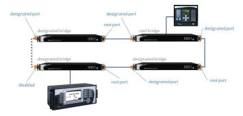
When using STP, only one path is available and transmits the network data. In the case of failure in any link between two Ethernet switches, the STP protocol recalculates the best path once again and after a short period of time the communication is reestablished. The time to recover the communication is also dependent on the STP protocol version.
