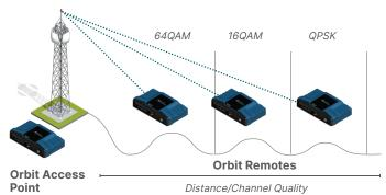
Bi-Directional Adaptive modulation maximizes throughput in both upstream and downstream directions for each remote independently. It enables Access Points and Remotes to transmit data at the highest possible modulation in real time, on a per-packet basis. The outcome is a network that does not sacrifice its overall performance for the least common denominator link.
