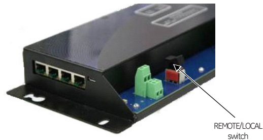
Figure 18: D20E-K REMOTE/LOCAL Switch
