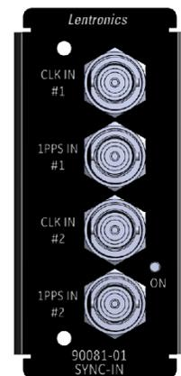
Left and Right CORE modules monitor for input via CLK IN #1 / 1PPS IN #1 and CLK IN #2 / 1PPS IN #2 respectively, enabling full redundancy. Secondary JPAX locations may be equipped with the Sync-IN unit to offer system-wide hardware redundancy, with fail over to internal timing supported upon complete loss of signal.
