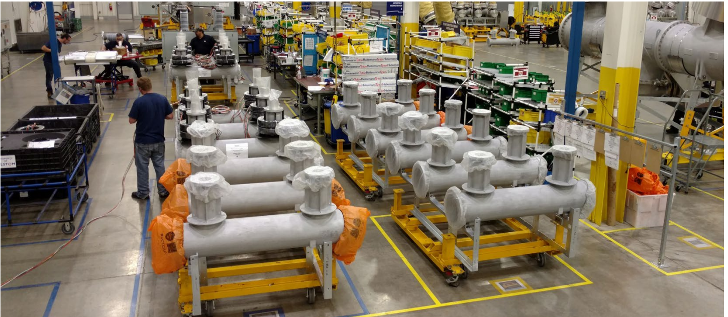
Dead Tank Circuit Breaker Assembly – installation of interrupters and current transformers to 72.5 kV dead tank circuit breakers.
