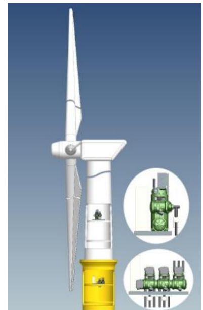
GIS split between tower and transition piece
